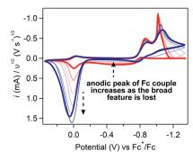
Fig. 9 Cyclic voltammograms of 10 mM  $[Ni(P^{Pn}_2N^{Pn}_2)_2]^{2+}$  with 1 mM ferrocene recorded at scan rates ranging from 0.025 (red) to 5 (dark blue) V s<sup>-1</sup>. All voltammograms obtained in 0.25 M  $[NBu_4][PF_6]$  acetonitrile using a glassy carbon working electrode and normalized to  $_{11}^{1/2}$
