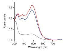
Fig. 5 UV-vis absorbance spectrum of a solution of 4 mM [Ni( $P^{Ph}_{2}$ - $N^{Ph}_{2}$ ) $_{2}$ | $^{2+}$  in 0.25 M [NBu $_{4}$ ][PF $_{6}$ ] acetonitrile during spectroelectrochemistry experiments. Spectra collected in the absence of an applied potential (blue), after holding the electrode at -1.4 V for 30 seconds (grey), and after stepping the fouled electrode to 0.3 V for 30 seconds (red). Double potential step chronoamperogram recorded with a platinum honeycomb electrode.
