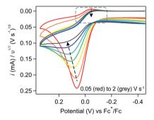
Fig. 12 Cyclic voltammograms of 5 mM [Ni(P<sup>Ph</sup><sub>2</sub>N<sup>Ph</sup><sub>2</sub>)<sub>2</sub>]<sup>2+</sup> with 0.1 mM Fc after a 5 second induction period at a resting potential of -1.5 V. Scan rate varied from 0.05 (red) 0.1 (orange), 0.2 (yellow), 0.3 (green), 0.5 (light blue), 1 (blue), and 2 (grey) V s<sup>-1</sup>. Voltammograms recorded in 0.25 M [NBu<sub>4</sub>][PF<sub>6</sub>] acetonitrile using a glassy carbon working electrode and normalized to  $v^{1/2}$
