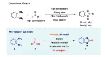
Scheme 1 Synthesis of benzimidazole and its derivatives by conventional methods<sup>22,23</sup> (above) and microdroplet synthesis (below).
