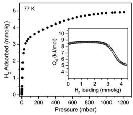
Fig. 2 Hydrogen adsorption isotherm for 1, measured at 77 K. Inset: loading-dependent isosteric heat of adsorption ( $Q_{st}$ ) for H<sub>2</sub> in 1.
