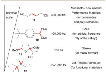
Fig. 2 Some electro-organic processes on the technical scale.
