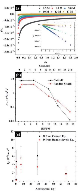
Fig. 4 Investigation of the diffusion coefficient of the ferro/ferri cyanide redox spices using 10 mM K<sub>3</sub>Fe(CN)<sub>6</sub> as a function of KF concentration (a) chronoamperometry, (b) diffusion coefficient, and (c) dependence of the heterogeneous electron transfer rate constant on electrolyte activity using reported KF activity coefficients. 40,41 Note the semi-logarithmic scale of (b).
