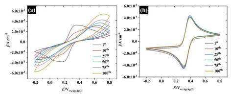
Fig. 6 Repeated CV cycles at 100 mV s<sup>-1</sup> at HOPG in 10 mM K<sub>₹</sub>Fe(CN)<sub>6</sub> using (a) 0.5 M KF, and (b) 17 M KF as supporting electrolytes.
