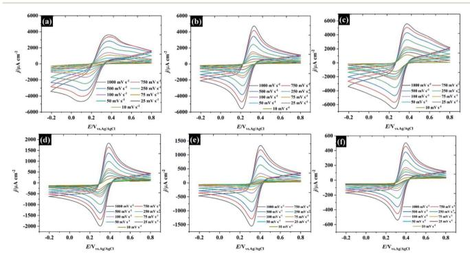
Fig. 3 CVs recorded using 10 mM  $K_3$ Fe(CN)<sub>6</sub> in potassium fluoride as a supporting electrolyte on an HOPG working electrode. KF concentrations are: (a) 0.5 M, (b) 1.0 M, (c) 5.0 M, (d) 10 M, (e) 13 M, and (f) 17 M.
