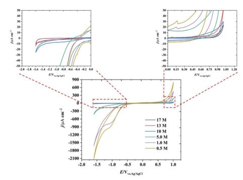
Fig. 1 CV of basal plane highly ordered pyrolytic graphite at  $1\,\mathrm{V}\,\mathrm{s}^{-1}$  as a function of KF concentration. The insets show the magnified response at the extremes of the potential range.
