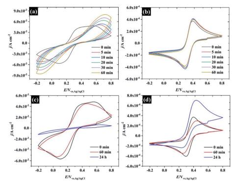
Fig. 7 CV of HOPG for the reduction of 10 mM Fe(CN)<sub>6</sub><sup>3-</sup> in aged KF electrolyte at a fixed concentration of (a) 0.5 M, and (b) 17 M. CV for the reduction of 10 mM Fe(CN) $_6^{3-}$  in air aged at a fixed concentration of (c) 0.5 M, and (d) 17 M.
