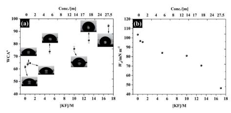
Fig. 8 Wettability of freshly cleaved highly ordered pyrolytic graphite (a) water in air contact angle at t = 0 s, and (b) work of adhesion as a function of KF concentration.
