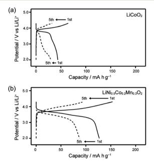
Fig. 8 Charge-discharge curves of Li half-cells composed of LC electrolyte 1/LiTFSI and various transition metal positive electrodes recorded at 80 °C; (a) LiCoO<sub>2</sub> and (b) LiNi<sub>0.5</sub>Co<sub>0.2</sub>Mn<sub>0.3</sub>O<sub>2</sub>.
