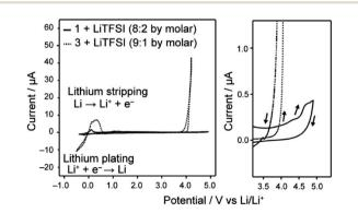
Fig. 3 Cyclic voltammograms of the LC electrolytes containing LiTFSI, recorded in the voltage region of -0.5–4.9 V vs. Li/Li<sup>+</sup> for 1/LiTFSI and -0.5–4.2 V vs. Li/Li<sup>+</sup> for 3/LiTFSI, respectively. Enlarged curves in the high voltage region are shown at the right part. Arrows in the right part indicate the sweep direction of cyclic voltammograms.
