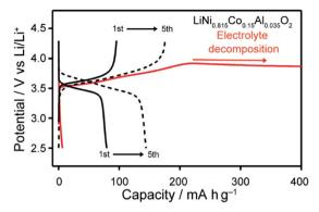
Fig. 9 Charge-discharge curves of Li half-cells composed of LC electrolytes of 1/LiTFSI (black) and 3/LiTFSI (red), and LiNi<sub>0.815</sub>Co<sub>0.15</sub>- $Al_{0.035}O_2$ , recorded at 80 °C
