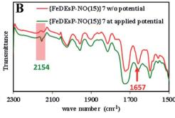
Fig. 8 Formation of N<sub>2</sub>O during the electrolysis of  $\{\text{FeDEsP-NO}\}^7$  at -1.31 V (vs. Fc<sup>+</sup>/Fc). On applying potential, N<sub>2</sub>O is generated ( $\nu_{\text{N-O}}_{(14/15)}$ : 2224/2154 cm<sup>-1</sup>), with the expense of  $\{\text{FeDEsP-NO}\}^7$  peaks ( $\nu_{\text{N-O}}_{(14/15)}$ : 1684/1657 cm<sup>-1</sup>): (A) in the presence of <sup>14</sup>NO and (B) in the presence of <sup>15</sup>NO.
