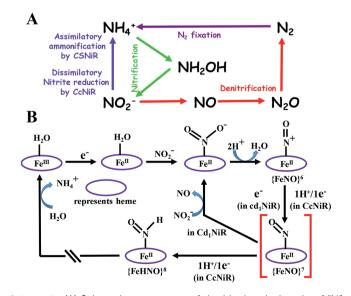
Scheme 1 (A) Selected components of the biochemical cycle of "N" and (B) proposed mechanistic pathways of nitrite reduction catalyzed by CcNiR and  $Cd_1NiR$ .<sup>2</sup>
