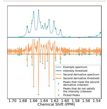
Fig. 3 Figure illustrating the gradient peak picking process. Peaks are picked if they are below a threshold in the second derivative (orange) and above an intensity threshold (blue). The final picked peaks are highlighted in green.
