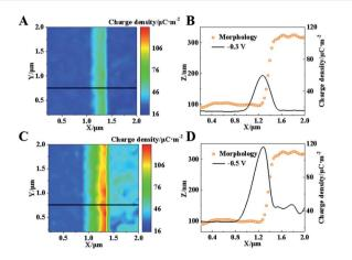
Fig. 4 (A) Charge density of the Pt–graphite interface at a voltage of -0.3 V. (B) Morphology and charge density along the black line in (A). (C) Charge density of the Pt–graphite step at a voltage of -0.5 V. (D) Morphology and charge density along the black line in (C).
