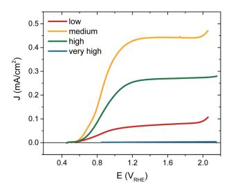
Fig. 3 Photocurrent responses for each WO $_3$  sample under simulated 1 sun illumination from the front side in 0.1 M H $_2$ SO $_4$ , scan rate 10 mV s $^{-1}$ . Data given for 'very high' [V $_0$ ] (blue), 'high' [V $_0$ ] (green), 'medium' [V $_0$ ] (yellow) and 'low' [V $_0$ ] (red).
