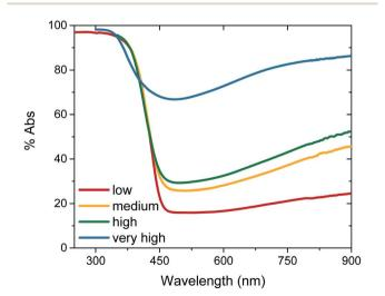
Fig. 1 UV-visible absorption spectra, determined from integrating sphere measurements of transmission and reflectance, for WO<sub>3</sub> films without annealing ('very high'  $[V_O]$ , blue), after acid treatment ('high'  $[V_O]$ , green), after 2 hour annealing ('medium'  $[V_O]$ , yellow) and after 12 hour annealing ('low'  $[V_O]$ , red).
