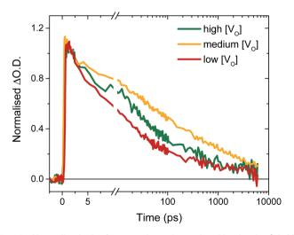
Fig. 5 Normalised ultrafast transient absorption kinetics in 0.1 M  $H_2SO_4$ , probing the electron decay at 700 nm from  $\sim\!200$  femtoseconds to 6 ns after excitation with 355 nm (0.2 mJ cm $^{-2}$ , no bias) for 'high' to 'medium' and 'low' [Vo] doping concentrations.
