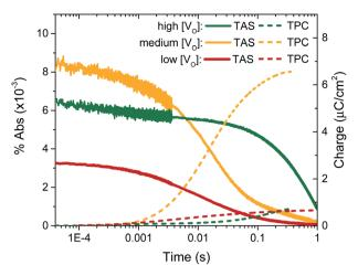
Fig. 4 Electron decays (solid lines, 800 nm) under bias (1.23  $V_{\rm RHE}$ ) from transient diffuse reflectance spectroscopy measurements in 0.1 M  $H_2SO_4$ , exciting at 355 nm with 0.25 mJ cm $^{-2}$ . The transient photocurrent was measured simultaneously and then integrated to give the transient charge collected (dashed lines). The high performing sample with 'medium' doping (yellow) is compared to samples of 'high' (green) and 'low' doping (red).
