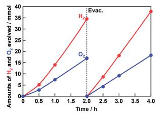
Fig. 4 Photocatalytic water splitting over  $Rh_{0.5}Cr_{1.5}O_3(0.2 \text{ wt}\%)/AgTaO_3$  under UV irradiation. Photocatalyst: 1 g, reactant solution: distilled water (340 mL), cell: inner-irradiation cell made of quartz, light source: 400 W high pressure Hg-lamp.  $AgTaO_3$  was synthesized by a solid state reaction at 1273 K for 15 h without excess Ag.  $Rh_{0.5}Cr_{1.5}O_3$  was loaded by an impregnation method at 623 K for 1 h.
