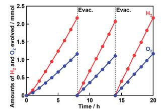
Fig. 1 Photocatalytic water splitting over  $Rh_{0.5}Cr_{1.5}O_3(0.2 \text{ wt%})/AgTaO_3$ . AgTaO<sub>3</sub> was synthesized by a solid state reaction at 1273 K for 15 h without excess Ag.  $Rh_{0.5}Cr_{1.5}O_3$  was loaded by an impregnation method at 623 K for 1 h. Photocatalyst: 0.3 g, reactant solution: distilled water (120 mL), cell: top-irradiation cell with a Pyrex window, light source: 300 W Xe-arc lamp ( $\lambda$  > 300 nm).
