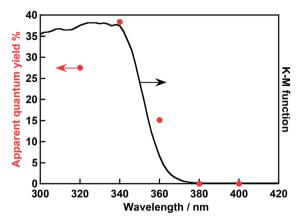
Fig. 3 An action spectrum of water splitting over  $Rh_{0.5}Cr_{1.5}O_3(0.2-wt\%)/AgTaO_3$  and a diffuse reflectance spectrum of  $AgTaO_3$  prepared by a solid state reaction at 1273 K for 15 h without excess Ag.  $Rh_{0.5}Cr_{1.5}O_3$  was loaded by an impregnation method at 623 K for 1 h. Photocatalyst: 0.3 g, reactant solution: distilled water (120 mL), cell: top-irradiation cell with a Pyrex window, light source: 300 W Xe-arc lamp with band-pass filters.
