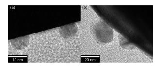
Fig. 2 TEM images of  $Rh_{0.5}Cr_{1.5}O_3(0.2 \text{ wt%})/AgTaO_3$  (a) before and (b) after photocatalytic water splitting under UV irradiation using a 300 W Xe-arc lamp.  $AgTaO_3$  was synthesized by a solid state reaction at 1273 K for 15 h without excess  $Ag. Rh_{0.5}Cr_{1.5}O_3$  was loaded by an impregnation method at 623 K for 1 h.
