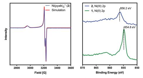
Fig. 2 (Left) Experimental (blue) and simulated (red) EPR spectra of 2 taken in  $CH_2Cl_2$ /toluene at 77 K. (Right) XPS spectrum of 2 (top) and 1 (bottom). The  $\sim$ 1 eV shift is consistent with a one-electron oxidation of the nickel center.
