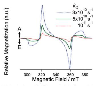
Fig. 7  $k_D$  dependence of the EPR spectra for the T + T state with J =0 computed by the sequential ESPT model (Fig. 6) via the intermediate T···T state.  $k_J$  was fixed to be  $10^{11}$  s<sup>-1</sup>.
