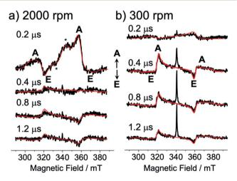
**Fig. 3** Delay time dependence of the TREPR spectra after the 532 nm laser irradiation of the as-spun TIPS-Pn thin films prepared with the spinning rates of (a) 2000 rpm and (b) 300 rpm. Detection temperature was 80 K. Computed EPR spectra (red lines) were obtained by spin polarization calculations of the correlated T + T (Fig. 4 and 5) by the electron spin polarization transfer with the quintet and singlet precursors causing A/E/A/E and E/A/E/A patterns (Fig. S2 $\dagger$ ), respectively.
