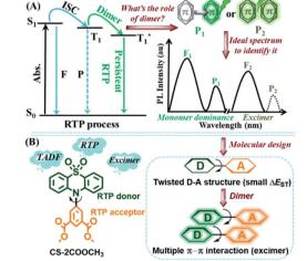
Fig. 1 (A) The query about the role of dimers in the persistent RTP effect and the proposed solution, in which F<sub>1</sub> indicates monomerdominated fluorescence, P1 indicates monomer-dominated RTP, F2 indicates singlet excimer fluorescence and P<sub>2</sub> indicates possible triplet excimer RTP. (B) The molecular structure and design strategy of CS-2COOCH<sub>3</sub>.
