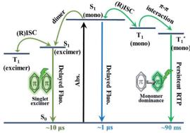
Fig. 6 The proposed PL process of CS-2COOCH<sub>3</sub>.
