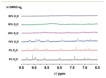
Fig. 6 Partial  $^{1}$ H NMR spectra of **5** in DMSO- $d_{6}$  upon increasing D<sub>2</sub>O content (IPt) =  $2.0 \times 10^{-4}$  M).
