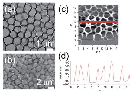
Fig. 2 (a) TEM and (b) SEM images of an air-dried sample of a dichloromethane solution of 1 ([Pt] =  $2.0 \times 10^{-4}$  M). (c) Tapping mode AFM image of an air-dried sample of a dichloromethane solution of 1 ( $[Pt] = 2.0 \times 10^{-4} \text{ M}$ ). (d) Height profile obtained along the red, solid line in the AFM image.
