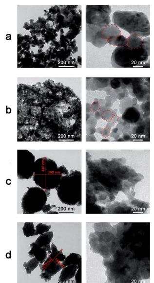
Fig. 9 Transmission electron microscope images of ZnO NPs synthesized at different pH values. (a) pH = 4. (b) pH = 6. (c) pH = 8. (d) pH = 10.
