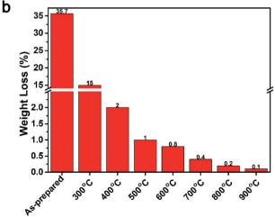
Fig. 6 Thermogravimetric analysis of the synthesized ZnO NPs for asprepared samples and for samples annealed at temperatures of 300-900 °C. (a) Thermogravimetric spectra. (b) Weight loss at 500 °C.
