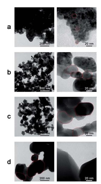
Fig. 4 Transmission electron microscope images of ZnO NPs with different annealing temperatures. (a) shows the as-prepared sample and (b), (c), and (d) show samples annealed at 400, 700, and 900 °C, respectively.
