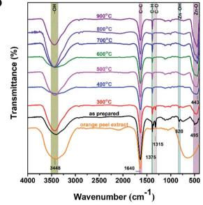
Fig. 5 The results of the synthesized ZnO NPs for as-prepared samples and for samples annealed at temperatures of 300-900 °C. (a) X-ray diffraction pattern. (b) Fourier-transform infrared spectroscopy.
