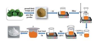
Fig. 1 Schematic diagram of the green synthesis of ZnO nanoparticles (ZnO NPs).
