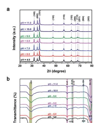
$\label{eq:Fig.10} \textbf{(a) X-ray diffraction patterns and (b) Fourier-transform infrared spectroscopy spectra of ZnO NPs synthesized at different pH values.}$
