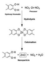
Fig. 2 The chemical mechanism of ZnO nanoparticle formation.
