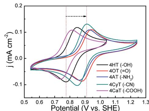
Fig. 1 CV curves of five TEMPO derivatives (1 mM) in 0.5 M KCl supporting electrolyte (pH = 7) at a scan rate of 25 mV s<sup>-1</sup> at 25  $^{\circ}$ C. Before CV measurements, the pH values of the electrolyte solutions were adjusted to 7 for 4AT and 4CaT by using 0.01 M HCl and KOH solution, respectively, because 4AT is weakly alkaline and 4CaT is weakly acidic.
