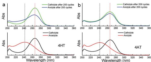
Fig. 7 Ultraviolet spectra of the anolyte and catholyte of the symmetric 4HT (a) and 4AT (b) RFBs, in  $2 \text{ M KCl}$  solution before and after 200 charge–discharge cycles.
