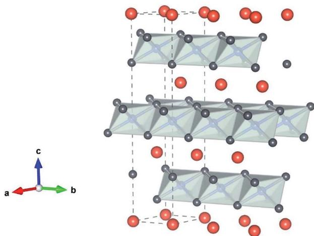
Fig. 2 The crystallographic framework of the layered LiMO<sub>2</sub> (M is Co or Ni) consisting of MO<sub>6</sub> octahedra (gray) and Li<sup>+</sup> (orange) "by VESTA".
