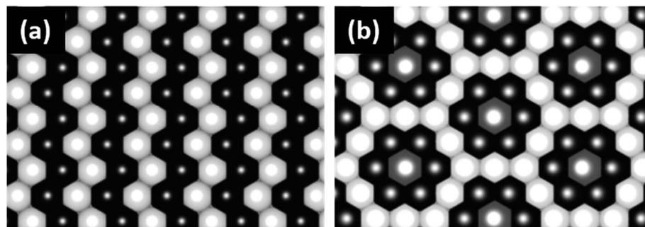
Fig. 7 (a) TM layer ordering of the flower structure and (b) transition metal layer ordering of the zigzag structure.<sup>59</sup>
