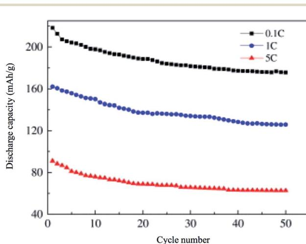
Fig. 17 Cyclic performance of nano C/ $\text{Li}_2\text{MnSiO}_4$  synthesized by ionothermal method, the material is tested in the potential range of 2.5–4.5 V.<sup>153</sup>
