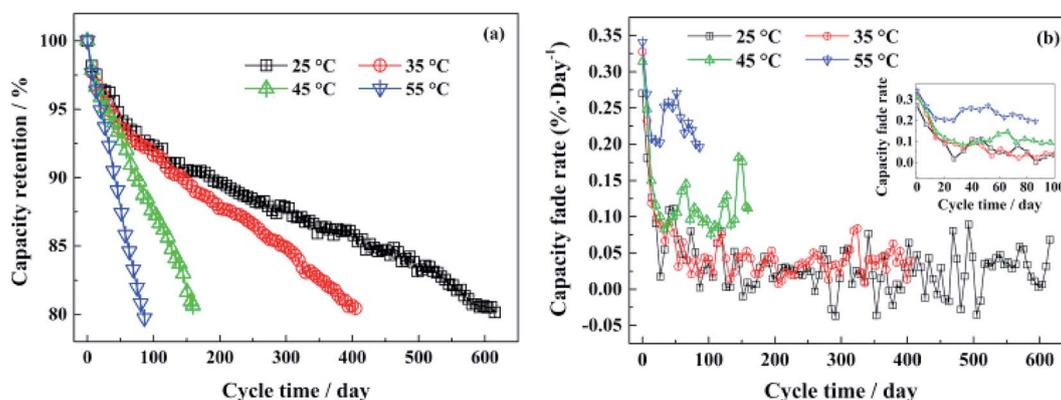
Fig. 10 (a) The capacity retentions of the LiFePO<sub>4</sub>/graphite full cells at different temperatures with continuous cycling days, (b) the capacity fade rate at each test temperature during cycling.<sup>113</sup>
