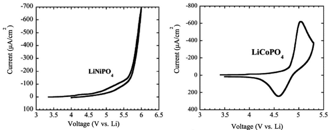
Fig. 14 Cyclic voltammetry of  $\text{LiNiPO}_4$  and  $\text{LiCoPO}_4$  at a scan rate of  $0.2 \text{ mV s}^{-1}$ .<sup>135</sup>
