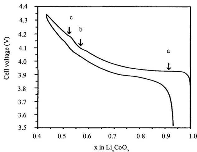
Fig. 3 Cell voltage of Li<sub>x</sub>CoO<sub>2</sub> as a function of *x*.<sup>12</sup>
