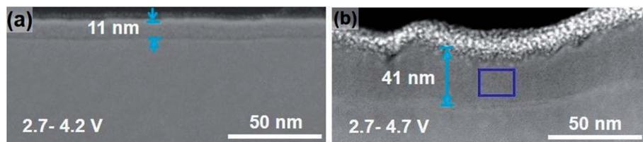
Fig. 5 Effect of high charge cutoff voltage on the thickness of the surface degradation layer.<sup>14</sup>
