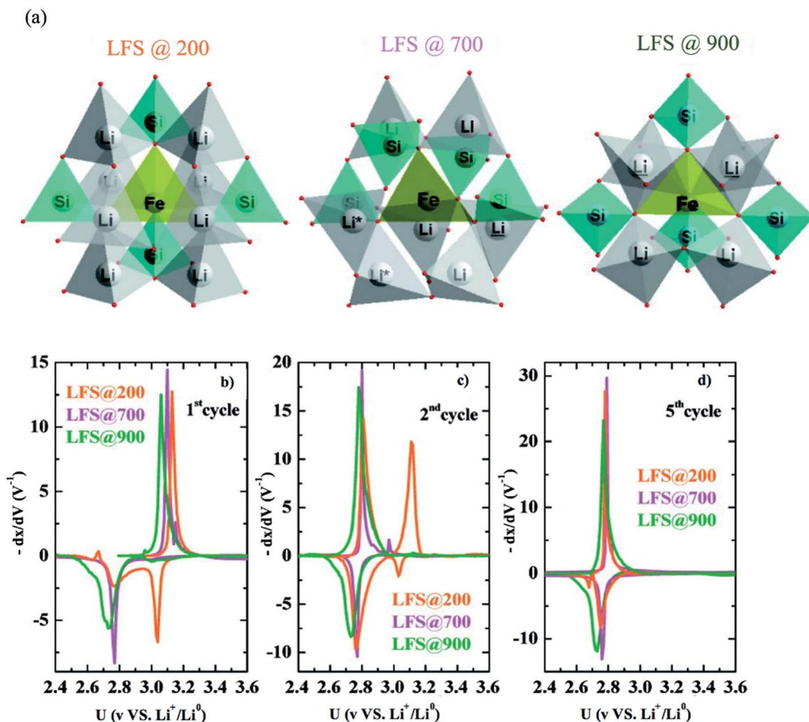
Fig. 15 (a) The three polymorphs of  $\text{Li}_2\text{FeSiO}_4$ , derivative plots obtained from PITT measurements in the (b) first, (c) second, and (d) fifth cycles for all three polymorphs.<sup>141</sup>
