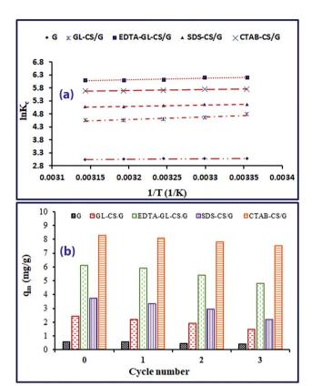
Fig. 8 Plots of  $\ln K_C versus 1/T$  for  $F^-$  ions adsorption on G, GL-CS/G, EDTA-GL-CS/G, SDS-CS/G and CTAB-CS/G adsorbents (a) and regeneration efficiency of the adsorbents (b).
