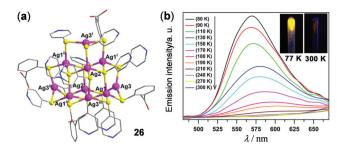
Fig. 22 (a) Crystal structure of the Ag-S hybrid cluster 26. (b) Temperature-dependent luminescence spectra of 26 in the solid state within the temperature range of 90-300 K. Inset: Photographs showing the emission color of 26 at 77 and 300 K under 365 nm irradiation. Reprinted with permission from ref. 76. Copyright 2017 Wiley-VCH.
