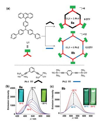
Fig. 7 (a) Synthetic routes and schematic diagram of metallacycles 8a and 8b. (b and c) Temperature-dependent emission spectral changes of (b) 8a in DMF and (c) 8b in THF ( $\lambda_{ex}$  = 400 nm, 2  $\times$  10  $^{-5}$  M). The insets show the emission colors at lower and higher temperature, respectively. Reprinted with permission from ref. 97. Copyright 2018 American Chemical Society.
