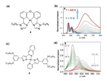
Fig. 4 (a) Molecular structure of Pt(II) complex 4. (b) Normalized temperature-dependent emission spectra of 4 in degassed Me-THF (1  $\times$  10<sup>-3</sup> M,  $\lambda_{ex}$  = 397 nm). Reprinted with permission from ref. 91. Copyright 2017 Wiley-VCH. (c) Molecular structure of Pt(II) complex 5. (d) Normalized temperature-dependent emission spectral changes of the PMMA film doped with 5 upon heating from 21 to 137.3 °C. Reprinted with permission from ref. 92. Copyright 2020 Elsevier Ltd.
