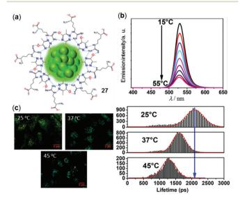
Fig. 23 (a) Chemical structural mode of Au NCs 27. (b) Temperaturedependent emission spectra of 27 in water in the range of 15-55 °C ( $\lambda_{\rm ex}$ = 375 nm). (c) Left: FLIM images of MG-63 cells with the internalized NCs 27 at 25, 37, and 45 °C. Right: Lifetime distribution histogram of intracellular NCs showing the changes in the lifetime and emission intensity at different temperatures. Reprinted with permission from ref. 122. Copyright 2019 American Chemical Society.
