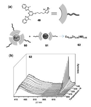
Fig. 37 (a) Molecular structures of 49-52. (b) Temperature-dependent emission spectra of 52 recorded from 80 to 500 K. Reprinted with permission from ref. 150. Copyright 2015 Wiley-VCH.
