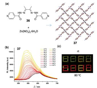
Fig. 30 (a) Schematic representation of the synthesis of 2D Zn(II) polymer 37. (b) Temperature-dependent solid-state emission spectra of 37 in the range of 27-95 °C. (c) Photographs under UV irradiation of 37 at ambient temperature and 80 °C, respectively. Reprinted with permission from ref. 133. Copyright 2020 The Royal Society of Chemistry.
