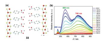
Fig. 27 (a) Structure representation of the 2D Cu-S polymer 33 viewed from the c axis. Orange, Cu; yellow, S; red, O; grey, C. Hydrogen atoms are omitted for clarity. (b) Temperature-dependent solid-state emission spectra of **33** between 93 and 503 K ( $\lambda_{\rm ex}$  = 380 nm). Reprinted with permission from ref. 129. Copyright 2016 The Royal Society of Chemistry.
