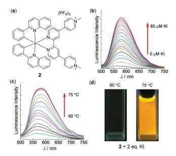
Fig. 2 (a) Molecular structure of Ir(III) complex 2. (b) Luminescence spectra change of 2 in degassed CH<sub> $\tau$ </sub>CN (1.0  $\times$  10<sup>-5</sup> M) at 75 °C with an increasing amount of KI from 0 to 10 equiv. (c) Temperature-dependent luminescence spectral change of 2 with 2 equiv. of KI upon heating from 60 to 75 °C. (d) Photographs of the solution of 2 at 60 or 75 °C in the presence of 2 equiv. of KI. Reprinted with permission from ref. 89. Copyright 2016 WILEY-VCH.
