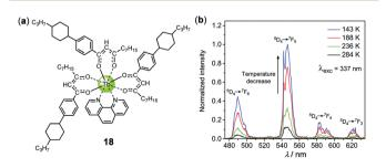
Fig. 17 (a) Molecular structure of Tb(III) complex 18. (b) Temperaturedependent time-delayed emission spectra of a film with a time delay of 2.5 µs. Reprinted with permission from ref. 107. Copyright 2018 The Royal Society of Chemistry.
