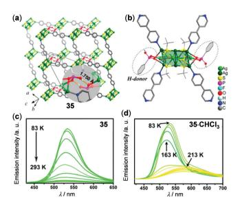
Fig. 29 (a) Two-layer stack and (b) perspective view of the coordination environment of Aq-MOF 35. (c and d) Temperature-dependent solidstate emission spectral change of (c) 35 and (d) 35·CHCl<sub>3</sub>. Reprinted with permission from ref. 131. Copyright 2018 American Chemical Society
