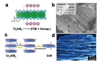
Fig. 11 (a) Crystal structures of Ti<sub>2</sub>InB<sub>2</sub>; (b) SEM image of the TiB phase. Reproduced with permission from ref. 79. Copyright 2019 Nature Publishing Group, 2018 Elsevier, respectively. (c) Schematic illustration of the transformation from Cr<sub>2</sub>AlB<sub>2</sub> to 2D-CrB. (d) SEM images of CrB nanosheets. Reproduced with permission from ref. 80. Copyright 2018 Elsevier, respectively.
