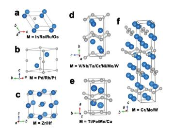
Fig. 4 Crystal structures of (a) WC-type monoboride; (b) anti-NiAstype monoboride; (c) NaCl-type monoboride; (d) CrB-type monoboride; (e) TiB-type monoboride; (f) MoB-type monoboride. Metal atoms and boron atoms are in blue and grey, respectively.
