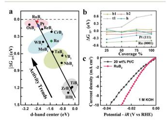
Fig. 13 (a) Fitted linear relationship between the adsorption free energy of atomic hydrogen ( $\Delta G_{H^*}$ ) and the d-band center of MB<sub>2</sub>, Pt and Ru. (b)  $\Delta G_{H^*}$  on the RuB<sub>2</sub>(001), Ru(0001) and Pt(111) surface as a function of hydrogen coverage. (c) LSV curves for RuB2 and 20 wt% Pt/C in 1.0 M KOH solution. Reproduced with permission from ref. 38. Copyright 2019 Wiley-VCH.
