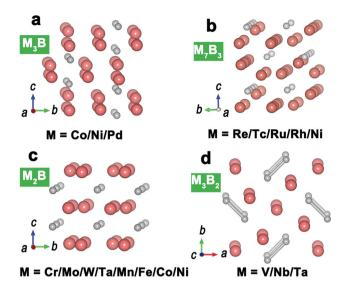
Fig. 3 Representative crystal structures of (a) M<sub>3</sub>B; (b) M<sub>7</sub>B<sub>3</sub>; (c) M<sub>2</sub>B; (d) M<sub>3</sub>B<sub>2</sub>. Metal atoms and boron atoms are in pink and grey, respectively.
