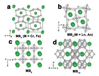
Fig. 6 Crystal structures of (a) MB<sub>4</sub> (M = Cr, Fe); (b) MB<sub>4</sub> (M = Y, La, Ce, Pr, Nd, Sm, Gd, Tb, Dy, Ho, Er, Tm, Yb, Lu, Th, U and Pu); (c) MB<sub>6</sub> (M = K, Ca, Sr, Ba, Y, La, Ce, Pr, Nd, Sm, Eu, Gd, Tb, Dy, Ho, Er and Tm); (d) MB<sub>12</sub> (M = Zr, Hf, Y, Gd, Tb, Dy, Ho, Er, Tm, Yb, Lu, Th, U and Pu). Metal atoms and boron atoms are in green and grey, respectively.
