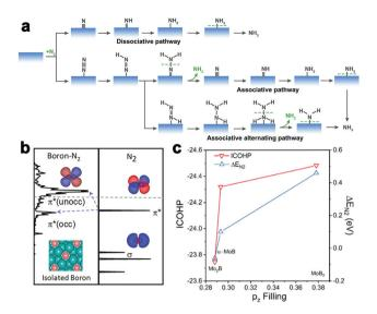
Fig. 16 (a) Schematic illustration of NRR reaction pathways on the catalyst surface. (b) Schematic illustrations of hybridization interactions between the boron p-orbital of Mo<sub>2</sub>B and the  $\pi^*$ -orbital of the N<sub>2</sub> molecule. (c) Correlation between pz-orbital filling with ICOHP and adsorption energy of N2. Reproduced with permission from ref. 46. Copyright 2020 the American Chemical Society.
