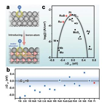
Fig. 14 (a) Schematic illustration of the influence of metal-boron orbital interaction on surface hydrogen adsorption properties in borides. (b) Calculated  $\Delta G_{H^*}$  values of fifteen monoborides and Pt. (c) A volcano plot presenting the exchange current densities for the HER as a function of  $\Delta G_{H^*}$  values for different materials. Reproduced with permission from ref. 41. Copyright 2020 Wiley-VCH.
