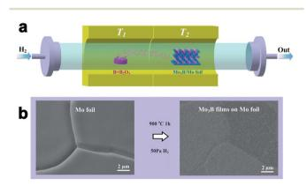
Fig. 9 (a) Schematic diagram of the growth of  $Mo_3B$  layers on Mo foils. (b) SEM images of the Mo foil before and after boronization. Reproduced with permission from ref. 73. Copyright 2017 Royal Society of Chemistry.
