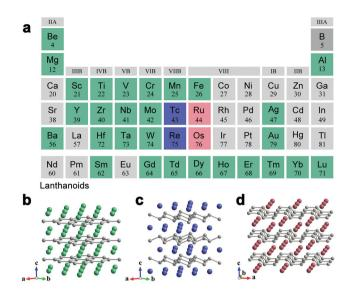
Fig. 5 (a) Elements constructing metal diborides. Crystal structures of (b) AlB2-type diboride; (c) ReB2-type diboride; (d) RuB2-type diboride. Boron is in grey, and metals used for constructing the AlB2-type, ReB2type and RuB<sub>2</sub>-type diborides are in green, blue and pink, respectively. Reproduced with permission from ref. 38. Copyright 2019 Wiley-VCH.
