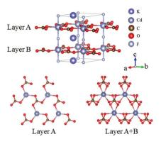
Fig. 17 The crystal structure of KCdCO<sub>3</sub>F, in which the [CO<sub>3</sub>] units in neighbouring [CdCO<sub>3</sub>] layers exhibit a small rotation.
