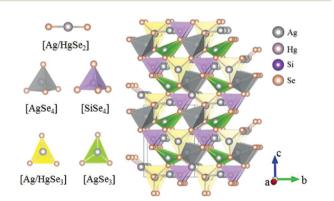
Fig. 26 Crystallographic structure of Ag<sub>6</sub>HgSiSe<sub>6</sub>.
