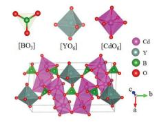
Fig. 14 Crystal structure of Cd<sub>4</sub>Y(BO<sub>3</sub>)<sub>3</sub>.
