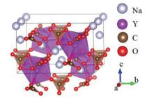
Fig. 15 The crystal structure of Na<sub>3</sub>Y(CO<sub>3</sub>)<sub>3</sub>.
