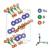
Fig. 28 Crystallographic structure of Na<sub>2</sub>BP<sub>2</sub>.
