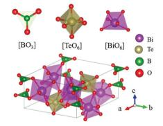
Fig. 24 The crystal structure of Bi<sub>3</sub>TeBO<sub>9</sub>
