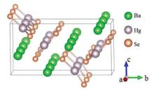
Fig. 25 Crystallographic structure of BaHgSe<sub>2</sub>.
