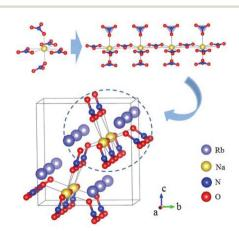
Fig. 18 Crystallographic structure of Rb<sub>2</sub>Na(NO<sub>3</sub>)<sub>3</sub>.
