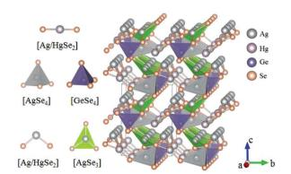
Fig. 27 Crystallographic structure of Ag<sub>6</sub>HgGeSe<sub>6</sub>.
