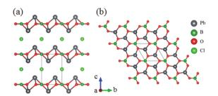
Fig. 13 (a) The crystal structure and (b) the [PbBO<sub>3</sub>] layer of Pb<sub>2</sub>BO<sub>3</sub>Cl.
