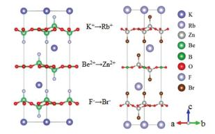
Fig. 12 Structural evolution from KBBF to RbZn<sub>2</sub>BO<sub>3</sub>Br<sub>2</sub>.
