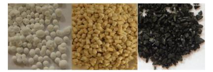
Fig. 4 The photographs of UiO-66-COOH beads obtained by freeze granulation (left) and extrudates (center), and of commercial type K adsorbent (activated carbon) from 3 M (right). Reprinted with permission from ref. 106. Copyright 2018 American Chemical Society.
