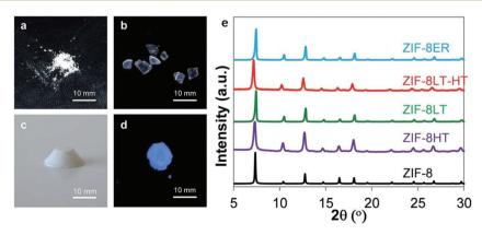
Fig. 12 (Left) Optical photos of (a) ZIF-8HT; (b) ZIF-8LT; (c) ZIF-8ER and (d) ZIF-8ER samples under 365 nm UV light. (e) PXRD patterns of the different ZIF-8 samples alongside a simulated pattern for ZIF-8. Adapted with permission from ref. 145 published by the Royal Society of Chemistry.
