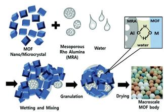
Fig. 2 The preparation of MOF granules/spheres through agglomeration of MOF and amorphous mesoporous alumina particles by a wet granulation technology. Reprinted with permission from ref. 54 published by the Royal Society of Chemistry.
