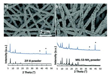
Fig. 17 SEM images and the corresponding XRD patterns of: (a) PAN/ZnO/ZIF-8 and (b) PAN/Al<sub>2</sub>O<sub>3</sub>/MIL-53-NH<sub>2</sub> composite materials; diffraction peaks of Al-foil are marked with (\*) and diffraction patterns of ZIF-8 and MIL-53-NH<sub>2</sub> reference powder samples are presented for comparison. Reprinted with permission from ref. 172 published by the Royal Society of Chemistry.
