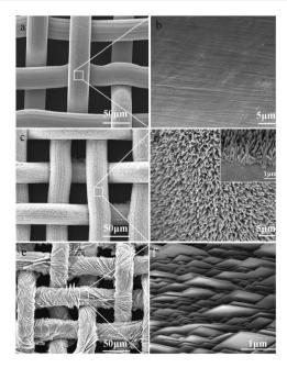
Fig. 19 SEM images of the bare stainless steel mesh (SSM) (a and b), ZnO nanorods grown on the SSM (c and d) and oriented Zn<sub>2</sub>(blm)<sub>4</sub> nanosheet grown on the SSM, SSM-500 (e and f). The inset is the cross section of the ZnO rods grown on the SSM. Reprinted with permission from ref. 82. Copyright 2019 Elsevier.
