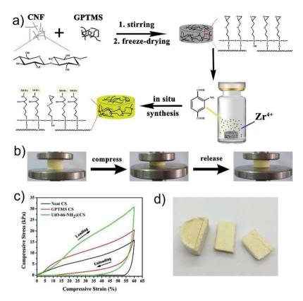
Fig. 15 (a) Schematic illustration for the preparation of a UiO-66-NH<sub>2</sub>-loaded cellulose sponge; (b) the photos of the MOF-loaded cellulose sponge during the compression process; (c) compressive stress-strain curves of neat cellulose sponge (CS), GPTMS modified cellulose sponge (GPTMS CS) and UiO-66-NH2-loaded cellulose sponge (UiO-66-NH2@CS); (d) a digital photograph of the UiO-66-NH2-loaded cellulose sponge. Reprinted with permission from ref. 164. Copyright 2019 Elsevier.
