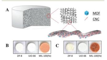
Fig. 8 (A) The schematic representation of a MOF-cellulose hybrid aerogel. Photographs of (B) CNC-CMC-MOF based hybrid aerogels (CNC:CMC:MOF = 1:1:1) by weight), and (C) all-CNC-MOF based hybrid aerogels (CNC: CNC: MOF = 1:1:1 by weight); aerogels are about 7 mm in diameter and 5 mm in height. Reprinted with permission from ref. 123. Copyright 2016 John Wiley and Sons.
