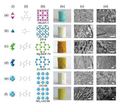
Fig. 10 The crystal structures of HKUST-1, ZIF-8, Mg-MOF-74, Zn-MOF-74, UIO-66, and NH<sub>2</sub>-UiO-66, and the optical photos and SEM images of the MOF@CMC foams based on these MOFs. The scale bars are 100 µm in v and 1 µm in vi. Reprinted with permission from ref. 133. Copyright 2016 American Chemical Society.
