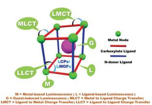
Scheme 1 Schematic representation for various pathways of luminescence origin in LCPs/LMOFs. 18,58
