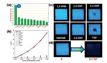
Fig. 2 (a) Quenching efficiency of (8) for different nitro analytes; (b) Stern-Volmer traces of various nitro analytes (0-200  $\mu$ L; 2 mM) in a water suspension of (8) (2 mg/2 mL); (c) digital photographs of paper strips coated with (8) after adding various nitro analytes under UV light (365 nm); (d) the paper strip dipped in 2 mM aqueous solution of TNP for 10 s showed full darkening of paper strip of (8). Reproduced with permission from ref. 70. Copyright 2016 Royal Society of Chemistry.
