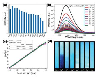
Fig. 9 (a) Emission quenching (%) of (13) upon addition of different cations; (b) emission behavior of (13) dispersed in water toward different concentrations of Hg<sup>2+</sup>; (c) Stern-Volmer plots for (13) upon gradual addition of Hg<sup>2+</sup> solution; (d) digital images of (13)-coated test strips after they were dipped in aqueous solutions of cations. Reproduced with permission from ref. 74. Copyright 2017 American Chemical Society.
