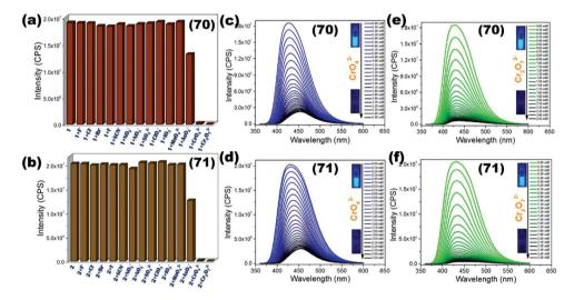
Fig. 11 (a and b) Fluorescence guenching effect of different agueous anion solutions on LMOFs (70) and (71); (c-f) luminescence titration of (70) and (71) by increasing concentration of  $CrO_4^{2-}/Cr_2O_7^{2-}$  solutions in water. Reproduced with permission from ref. 120. Copyright 2017 American Chemical Society.
