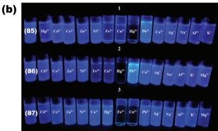
Fig. 12 (a) Quenching percentage of (85-87) in the presence of different metal ion solutions, (b) digital images blank (85-87) and after addition of different metal ion solutions under UV light (310 nm). Reproduced with permission from ref. 126. Copyright 2018 American Chemical Society.
