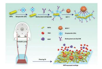
Fig. 9 Illustration of a multifunctional coating of HNTs on the inner surface of microtubes for specific capture of circulating tumor cells (MCF-7, human breast adenocarcinoma) in real blood samples. The HNTs increase the active surface for cell capture and serve as an anchorage for specific anti-EpCAM antibody *via* biotin-streptavidin interactions. RBC = red blood cells, WBC = white blood cells. Reproduced from ref. 154. Copyright 2018, with permission from Elsevier.
