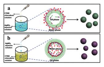
**Fig. 9** Schematic explanation for the one-pot surfactant-assisted synthesis of Ag/AgBr-based nanostructures *via* an oil/water (a) and a water/oil (b) microemulsion system. Copyright 2012, American Chemical Society. Reprinted from ref. 84 with permission.
