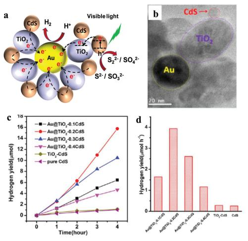
Fig. 5 (a) Schematic illustration of photocatalytic activity of the Au@TiO2-CdS nanocomposite, (b) TEM, (c) plots of the photocatalytic HER versus visible light irradiation time and (d) HER for pristine CdS, binary TiO<sub>2</sub>-CdS and various ternary nanocomposites. Fig. 4b-d: Copyright 2013, American Chemical Society. Reprinted from ref. 35 with permission.
