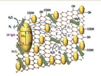
Fig. 1 Schematic illustration of photocatalytic activity of the TiO<sub>2</sub>/ MoS<sub>2</sub>/graphene nanocomposite.
