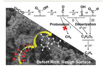
Fig. 6 Proposed pathway for the electroreduction of CO<sub>2</sub> to ethylene on the Re-Cu@Cu2(OH)3NO3 electrode.
