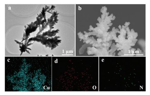
Fig. 3 (a) TEM and (b) SEM images and the corresponding elemental mapping images of (c) Cu, (d) O, and (e) N of the Re-Cu@Cu<sub>2</sub>(OH)<sub>3</sub>NO<sub>3</sub> electrode
