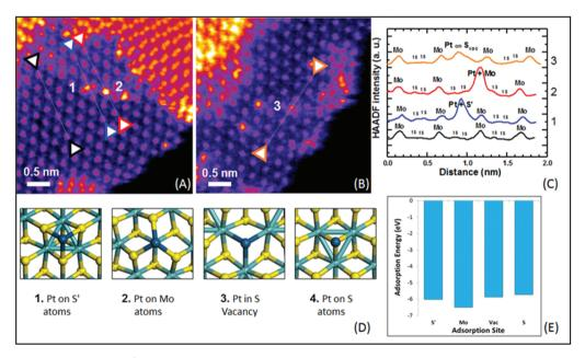
Fig. 4 (a) and (b) HAADF-STEM of Pt-1T- $^{S}MOS_2$ . (c) ADF intensity line profiles taken along the corresponding coloured line of black, blue, red, and orange in the  $\langle 110 \rangle$  direction. (d) The proposed model of the Pt atom doping at 4 different adsorption sites. Numbers 1, 2 and 3 correspond to the experimentally observed Pd position shown in (a) and (b). (e) Adsorption energy for Pt atoms on each proposed adsorption site. <sup>29</sup>
