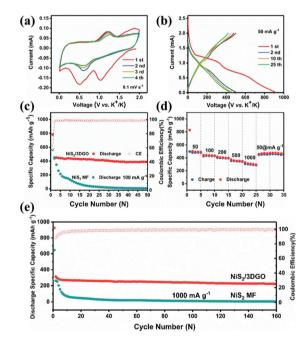
Fig. 4 (a) CV test result for the initial four cycles of NiS<sub>2</sub>/3DGO at 0.1 mV s<sup>-1</sup>. (b) Representative galvanostatic discharge/charge curves of  $NiS_2/3DGO$  at 50 mA  $g^{-1}$ . (c) Cycling performance of  $NiS_2/3DGO$  and NiS<sub>2</sub> MF at 100 mA g<sup>-1</sup>. (d) Rate performance of NiS<sub>2</sub>/3DGO at a different density. (e) Long-term cycling stability of NiS2/3DGO at  $1000 \text{ mA g}^{-1}$
