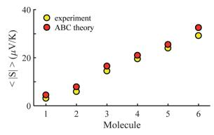
Fig. 4 Experimental and ABC-theory predictions for average of the magnitudes of Seebeck coefficients  $\langle |S| \rangle$  (yellow- and red-circles respectively).
