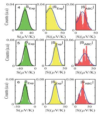
Fig. 3 Experimentally derived and predicted ABC theory histograms along with their Gaussian and folded fit curves (black- and blue-solid lines) for molecules 1–6. Experiment, folded experiment and predicted ABC theory Seebeck coefficients (green, yellow and red, left to right).
