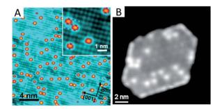
Fig. 3 (A) Au single atoms stabilized by monolayered CuO on a Cu(110) single crystal. Reproduced with permission.<sup>56</sup> Copyright 2018, American Chemical Society. (B) K single atoms stabilized by monolayered ceria on a Pt(111) single crystal. Reproduced with permission.<sup>57</sup> Copyright 2019, American Institute of Physics.
