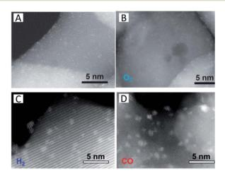
Fig. 2 (A) HAADF-STEM images of the as-prepared 1.66 wt% Pt<sub>1</sub>/  $Fe_2O_3$  SAC and the samples treated in (B)  $O_2$ , (C)  $H_2$ , and (D) CO at 250  $^{\circ}\text{C}$  for 2 h. Reproduced with permission.  $^{50}$  Copyright 2018, IOP Publishing Ltd.
