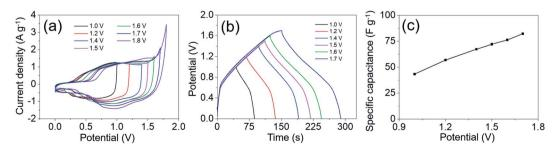
Fig. 11 (a) CV curves of the  $MgCo_2O_4$  NFs//AC ASC measured over different voltage windows at a scan rate of 10 mV s<sup>-1</sup>, (b) GCD curves of the  $MgCo_2O_4$  NFs//AC ASC measured over different voltage windows at a current density of 1 A g<sup>-1</sup>, and (c) specific capacitance as a function of voltage windows.
