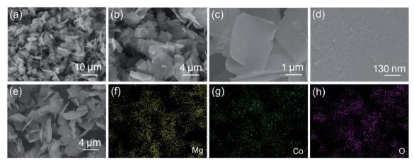
Fig. 2 (a-d) SEM images of  $MgCo_2O_4$  NFs obtained in the typical synthesis with a post annealing process in air, and (e-h) SEM image of  $MgCo_2O_4$  NFs and the corresponding elemental mapping images of Mg, Co, and O elements, respectively.
