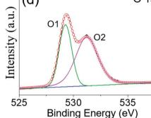
Fig. 4 (a) XPS survey spectrum and high-resolution spectra for (b) Mg 1s, (c) Co 2p, and (d) O 1s of the MgCo<sub>2</sub>O<sub>4</sub> NFs.
