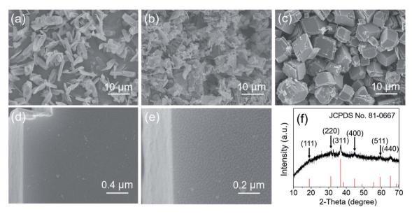
Fig. 6 SEM image of the MgCo<sub>2</sub>O<sub>4</sub> samples prepared at (a) 105, (b) 135, and (c-e) 150  $^{\circ}$ C, respectively, and (f) the XRD pattern of the MgCo<sub>2</sub>O<sub>4</sub> cubes. All the samples were annealed at 400  $^{\circ}$ C for 3 h.
