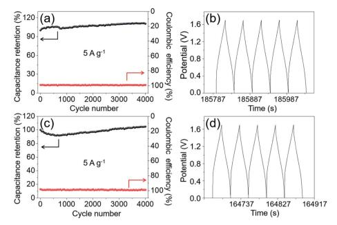
Fig. 13 (a) Consecutive 4000 cycle GCD curves at 5 A  $\rm g^{-1}$  and the related coulombic efficiency, and (b) the last 5 GCD curves of the MgCo<sub>2</sub>O<sub>4</sub> NFs//AC ASC, (c) continuous 4000 cycle GCD curves at 5 A  $g^{-1}$  and the related coulombic efficiency, and (d) the last 5 GCD curves of the MgCo<sub>2</sub>O<sub>4</sub> NCs//AC ASC.
