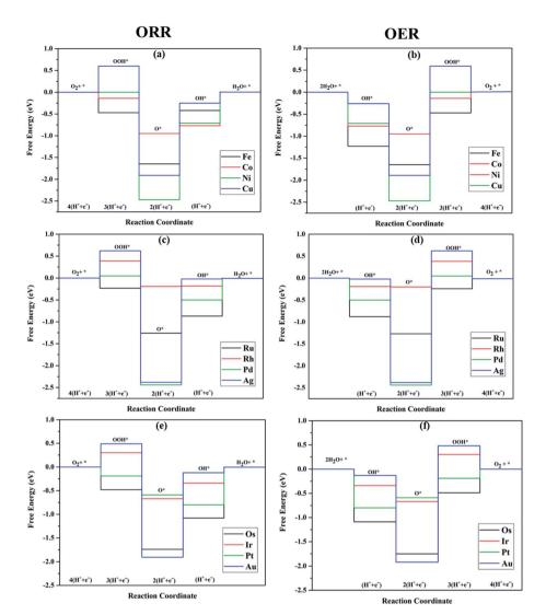
Fig. 6 Free energy diagrams of ORR and OER along the TM-Ph SAC series constructed at 1.23 V.
