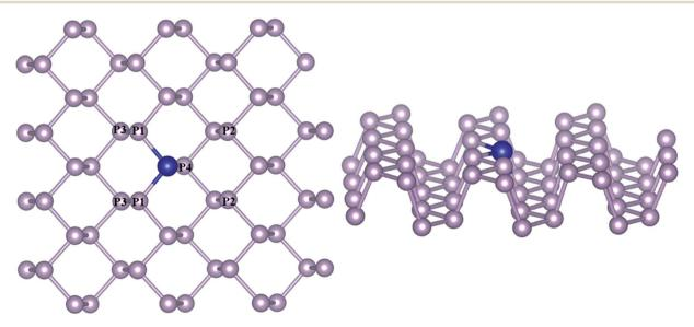
Fig. 1 Transition metal-doped phosphorene model (a) top view and (b) side view. P atoms differing in coordination with respect to the TM atom are labeled. Blue and violet colors represent the TM and P atoms, respectively.
