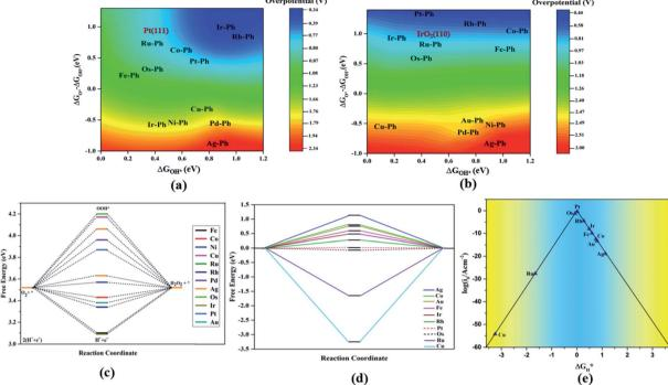
Fig. 7 (a and b) Two-dimensional ORR (a) and OER (b) activity volcano plots. The activities of the Pt(111) and IrO<sub>2</sub>(110) reference systems calculated at the GGA-RPBE level are shown in brown. (c) Free energy analysis of 2e<sup>-</sup> reduction by TM-Ph SACs at 0.7 V. (d) HER free energy diagram of TM-Ph SACs. (e) Current density volcano plot of HER vs.  $\Delta G_{H^*}$ .
