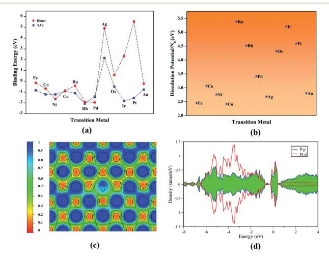
Fig. 2 (a) Binding energy trends of transition metal single atoms and dimers. (b) Dissolution potential of SACs per number of protons ( $N_H$ ). (c) Electron localization function and (d) Projected density of states of prototype Pt-Ph system.
