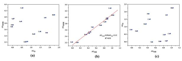
Scaling relationship of the ORR/OER intermediates, (a)  $\Delta G_{O^*}$  vs.  $\Delta G_{OH^*}$ , (b)  $\Delta G_{OOH^*}$  vs.  $\Delta G_{OH^*}$ , (c)  $\Delta G_{O^*}$  vs.  $\Delta G_{OOH^*}$ .
