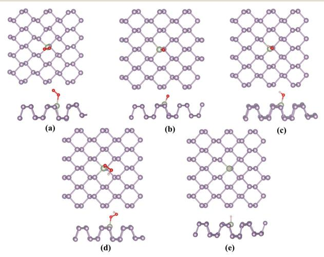
Fig. 3 Most stable adsorption configurations of the ORR/OER/HER intermediates, (a) O<sub>2</sub>, (b) O\*, (c) OH\*, (d) OOH\* and (e) H\*.
