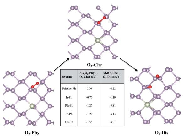
Fig. 8 Free energy analysis of O<sub>2</sub> interaction with TM-Ph SACs. Pristine phosphorene is the reference system. O<sub>2</sub>-Phy, O<sub>2</sub>-Che, and O<sub>2</sub>-Dis represent the physisorbed, chemisorbed and dissociated oxygen molecule, respectively.
