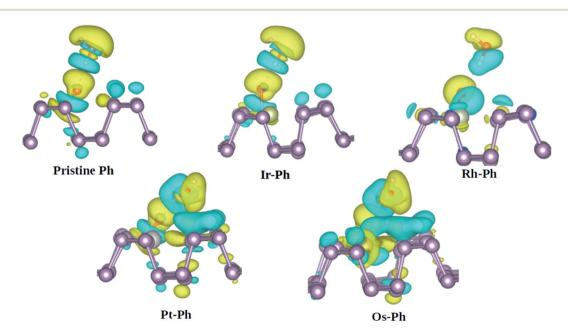
Fig. 9 Charge density difference analysis of  $H_2O$  with the  $O^*$ -bonded TM-Ph SACs and pristine phosphorene. Yellow and cyan colors represent the positive and negative isosurfaces, respectively, at 0.003 eV.
