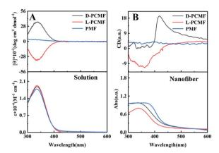
Fig. 3 CD and UV-vis absorption spectra of fluorescent polymers: (A) the spectra were measured in  $CHCl_3$  solution, and the concentration of the samples was 0.25 mM; (B) the spectra were qualitatively measured using electrospun nanofiber membranes infiltrated with toluene (a drop of toluene added on a circular membrane with a diameter of 1 cm). All the spectra were measured at room temperature.
