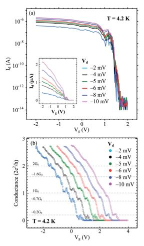
Fig. 8 (a) Transfer characteristics on the logarithmic scale of the devices fabricated from the Ge-core/a-Si shell nanowire with a channel length of 500 nm at low  $V_{\rm d}$  (-2, -4, -5, -6, -8 and -10 mV) at T=4.2 K. Inset: transfer characteristics on the linear scale. (b) Extracted conductances from (a) showing stepwise features at several  $G_0$  values including the quantization at  $\sim$ 0.7 $G_0$  ("0.7 structure"). The x-axis has been shifted to the right for clarity of comparison.
