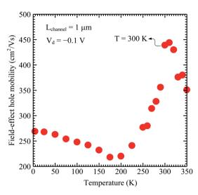
Fig. 7 Field-effect hole mobility *versus* temperature calculated at  $V_{\rm d}=-0.1$  V. The field-effect hole mobility value was selected at  $V_{\rm g}$  0.88 V for each temperature condition.
