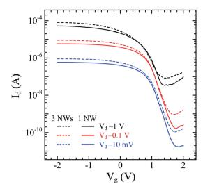
Fig. 5 Transfer characteristics ( $I_d$  versus  $V_g$  curve) of the devices consisting of a single nanowire (solid curves) and three nanowires (dashed curves) at a  $V_d$  of -0.01 V, -0.1 V and -1 V. The gate voltage ( $V_o$ ) was swept from -2 to 2 V. The channel length is 1  $\mu$ m.
