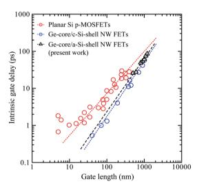
**Fig. 6** Intrinsic device speed or gate delay of Ge-core/a-Si shell nanowire FETs *versus* gate length. Planar Si p-MOSFETs from ref. 14 and Ge-core/crystalline Si-shell nanowire FETs from ref. 17 are included for comparison.
