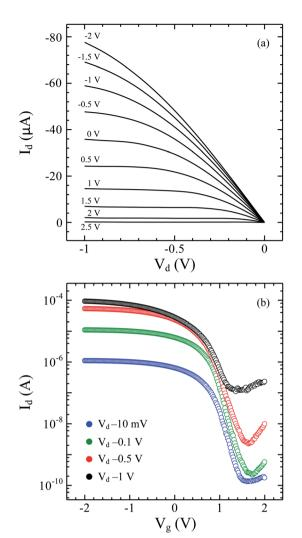
Fig. 2 (a). Output characteristics ( $l_{\rm d}$  versus  $V_{\rm d}$  curve) of the device fabricated from the Ge-core/a-Si shell nanowire with  $V_{\rm g}=2$  to -2.5 V in steps of 0.5 V from the top to the bottom. (b) Transfer characteristics ( $l_{\rm d}$  versus  $V_{\rm g}$  curve) of the device at  $V_{\rm d}=-0.01$ , -0.1, -0.5 and -1 V. The gate voltage ( $V_{\rm g}$ ) was swept from -2 to 2 V. The channel length is 800 nm.
