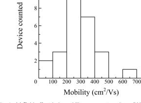
Fig. 4 (a) Field-effect hole mobility *versus* gate voltage ( $V_{\rm g}$ ) at  $V_{\rm d}=-0.01,\ -0.1,\ -0.5$  and -1 V. (b) Histogram of Ge-core/a-Si shell nanowire FET mobility.
