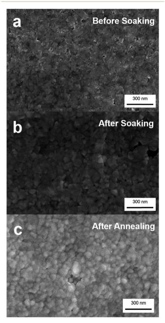
Fig. 2 Scanning electron microscope (SEM) images of (a)  $Cu_{2-x}$ Se thin film sample before soaking (b) Ag<sub>2</sub>Se thin film after soaking and (c) the Ag<sub>2</sub>Se sample post annealing. The images demonstrate the nanocrystalline grain structure as well as the continuous void-free nature of the  $Cu_{2-x}Se$  and the  $Ag_2Se$  films. Annealing does not significantly affect the average grain size of the Ag<sub>2</sub>Se film.
