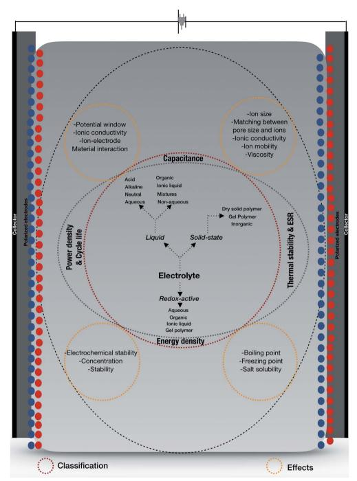
Fig. 9 Classification of electrolytes with electrochemical supercapacitor effects based on electrolytes.
