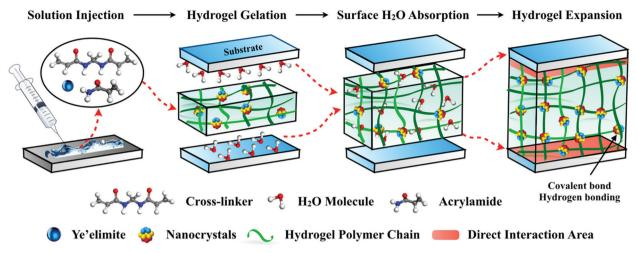
Fig. 1 Design of nanocrystal reinforced hydrogel networks. The monomer, crosslinker, and ye'elimite were simply blended to fabricate a nanocomposite PAM hydrogel solution, which was directly injected under water to the substrates. During gelation, the water molecules at the interfaces were captured into the hydrogel matrix, forming a sound bonding between the adhesives and the substrates.
