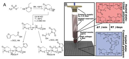
Fig. 1 (A) Synthesis of the furan and maleimide functionalized poly(2-ethyl-2-oxazine) (PEtOzi-M, PEtOzi-F) used in this study (DCC: dicyclohexyl carbodiimide, AN: acetonitrile, BN: benzonitrile). (B) Schematic illustration of the MEW setup, processing conditions and the reversible DA equilibrium allowing liquefaction and melt processing at elevated temperatures followed by the chemically crosslinking upon cooling.
