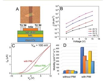
Fig. 4 (A) Schematic of the InSe-based FET device and the top-view optical microscopy image. (B) Leakage current density as a function of voltage in a capacitor device. (C) The  $I_{\rm ds} - V_{\rm g}$  transfer curve and (D) comparison of electron mobility in InSe for the FET devices with and without SO<sub>2</sub>-PIM. Five devices were tested for each type of FET.
