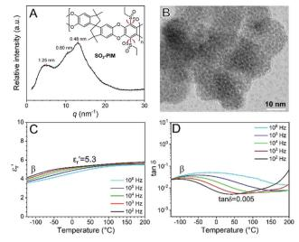
Fig. 1 (A) One-dimensional WAXD profile for the as-cast SO<sub>2</sub>-PIM (the chemical structure is in the inset). (B) Bright-field TEM micrograph of SO<sub>2</sub>-PIM stained by RuO<sub>4</sub> for 10 min. Temperature-scan BDS results of (C) the real part of the relative permittivity  $(\varepsilon_r)$  and (D) tan  $\delta$  at different frequencies.
