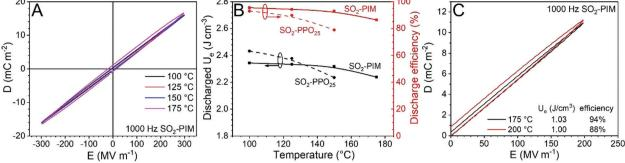
Fig. 3 (A) Bipolar D-E loops at high temperatures for  $SO_2$ -PIM. (B) Tempearture-dependent discharged energy density ( $U_e$ ) and discharge efficiency for SO<sub>2</sub>-PIM and SO<sub>2</sub>-PPO under 300 MV m<sup>-1</sup>. (C) Unipolar D-E loops under 200 MV m<sup>-1</sup> for SO<sub>2</sub>-PIM at 175 and 200 °C, respectively.
