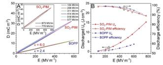
Fig. 2 (A) Unipolar D-E loops for  $SO_2$ -PIM under 1 kHz at room temperature. (B) Discharged energy density ( $U_e$ ) and discharge efficiencies as a function of the poling field for  $SO_2$ -PIM. BOPP is used for comparison.
