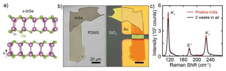
Fig. 1 Layered semiconducting ε-InSe. (a) Crystal structure of InSe. (b) Optical pictures of few-layer InSe exfoliated onto PDMS (left) and deterministically transferred onto pre-patterned gold electrodes (right). (c) Raman spectra (532 nm laser, power density 0.11 mW  $\mu$ m<sup>-2</sup>) of the InSe flake shown in panel b recorded in the pristine state and after two weeks in air conditions.
