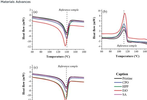
Fig. 3 DSC curves for the three cycles (a) first heating cycle, (b) cooling cycle and (c) second heating cycle for the set of samples.
