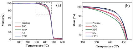
Fig. 5 TGA thermograms for the set of samples (a) from initial mass to its full degradation and (b) the threshold for the diverging mass loss rates, amplified from inset in (a).
