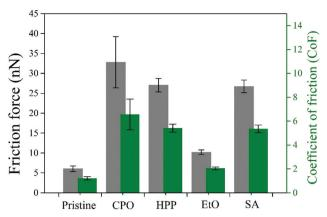
Fig. 8 Friction forces and coefficients for the studied conditions.
