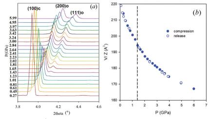
Fig. 1 Experimental XRD patterns ( $\lambda = 0.41116 \text{ Å}$ ) across the (100) reflection of the parent cubic phase as a function of pressure (reported in GPa on the left) (a) and corresponding lattice volume trend as a function of pressure (b). Dashed line highlights phase transition (see text for details).
