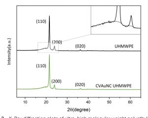
Fig. 2 X-Ray diffraction plots of ultra-high molecular weight polyethylene control and crystal violet gold nanocluster embedded ultra-high molecular weight polyethylene sample measured across  $2\theta$  range from 6 to 66°. A small section of the diffraction pattern of the UHMWPE was shown by a zoomed inset shown on the top right.
