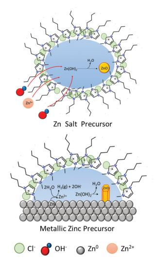
Fig. 8 Schematic of ZnO formation in  $[C_4C_1im]Cl$  at low water content. Left: Zn salts as precursors.<sup>40</sup> Right: Metallic zinc as precursor.
