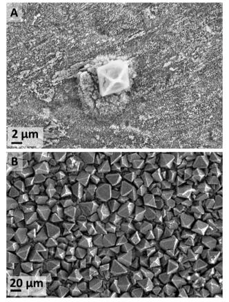
Fig. 3 SEM image showing zinc surface exposed to  $[C_4C_1im]Cl$  (IL-1,  $X_{\rm H_2O}$  = 0.98 solution at 20  $\pm$  1 °C). (A) Single octahedron Zn(OH)<sub>2</sub> particle after 18 d exposure (approximate length of 7.9  $\pm$  0.6  $\mu$ m). (B) Multiple Zn(OH)<sub>2</sub> crystals after 44 d exposure with a mean length of 21  $\pm$  6  $\mu$ m (n = 84).
