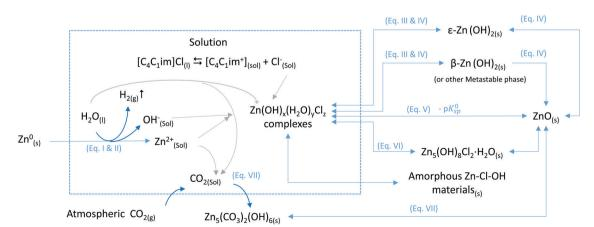
Fig. 9 General conversion paths of metallic zinc into ZnO in  $[C_4C_1\text{im}]Cl$ /water systems. Equations in the scheme are not balanced. Equations are given in the text. The predominant path and species formed will depend on the temperature and water content.
