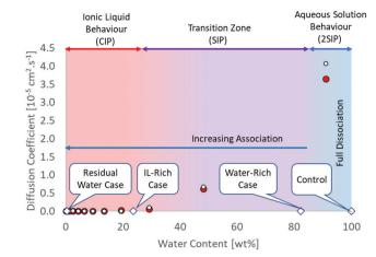
Fig. 1 Structural and diffusion properties of [C<sub>4</sub>C<sub>1</sub>im]Cl/water mixtures as a function of water concentration. Diffusion data calculated from MD simulations at 350 K.<sup>35</sup> White circle ( $\bullet$ ) chloride, red circle ( $\bullet$ ) [C<sub>4</sub>C<sub>1</sub>im<sup>+</sup>].
