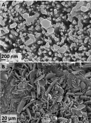
Fig. 4 Magnified zinc surface exposed to  $[C_4C_1im]Cl$  (IL-1,  $X_{H_2O} = 0.98$ solution at 70  $\pm$  1 °C). (A) ZnO nanorods after 4 d exposure (magnification 134.17k×) (average size 90  $\pm$  40 nm, n = 361). (B) ZHC plate-like crystals after 15 d exposure (magnification 1.44k×). Estimated thickness  $2.5 \pm 1.5 \; \mu \text{m} \; (n = 85), \; \text{diameter 19} \pm 8 \; \mu \text{m} \; (n = 85).$
