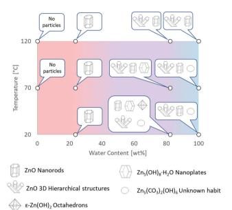
Fig. 2 Graphical summary of Zn-based materials, obtained by direct oxidation of metallic zinc in  $[C_4C_1im]Cl$  solutions, as a function of experimental conditions. Further details are provided in Tables S1 and S2 in ESI.†
