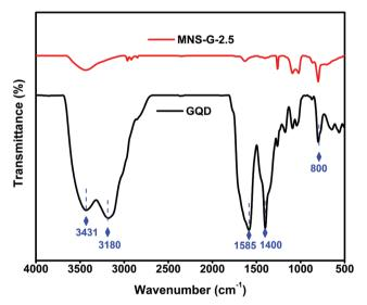
Fig. 5 FT-IR spectra of GQD and MNS-G-2.5.
