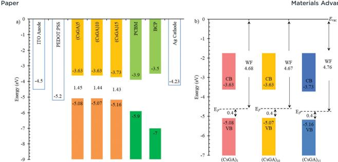
Fig. 4 (a) Band energy diagram of PVSCs with  $(CsGA)_x + 1.5\%$  EDAl<sub>2</sub> active layers, where x = 5, 10 and 15. The band gaps derived from the UV-Vis spectra are indicated. (b) Energy level scheme for the (CsGA)<sub>5</sub>, (CsGA)<sub>10</sub> and (CsGA)<sub>15</sub> films with 1.5% EDAI<sub>2</sub> based on the parameters derived from the UPS spectra
