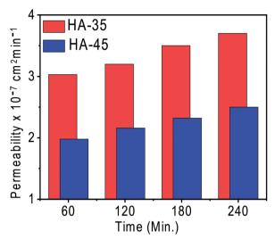
Fig. 3 Vanadium permeability for the prepared membranes.
