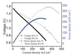
Fig. 7 Polarization curve for the prepared membranes.
