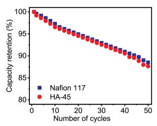
Fig. 8 Number of cycles *versus* capacity retention for HA-45 and Nafion 117 membranes
