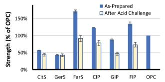
Compressive strength of terpenoid-sulfur composites (CitS, GerS, and FarS), ordinary Portland cement (OPC) and composite-infused cement (CIP, GIP, and FIP) measures before (blue bars) and after (yellow bars) being submerged in 0.5 M H<sub>2</sub>SO<sub>4</sub> for 24 h. OPC deteriorates after acid challenge so its post-acid strength could not be determined. Each measured value is an average of three trials, and the error bars represent the standard deviation of the three runs
