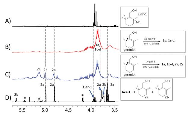
Fig. 2 Proton NMR spectra (CDCl<sub>3</sub>, 300 MHz) for (A) isolated **Ger-1**, (B) product mixture resulting from the reaction of geraniol with  $\geq$ 2 equiv. S, (C) product mixture resulting from the reaction of geraniol with 1 equiv. S, and (D) literature spectrum for a mixture of geraniol (peaks marked with asterisks), **2a** and **2b**. Spectra (A) and (D) are reprinted from reference  $^{1}$  ©2005, with permission from John Wiley and Sons.
