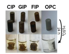
Fig. 5 Appearance of terpenoid–sulfur composite (A) or of ordinary portland cement (OPC) and composite-infused portland cement (B) compressional test cylinders before and after submersion in  $0.5 \, \mathrm{M} \, \mathrm{H}_2 \mathrm{SO}_4$  for 24 h.
