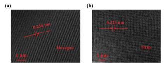
Fig. 3 (a and b) Lattice fringes of different  $CH_3NH_3PbI_3$  perovskite crystals characterized by TEM.
