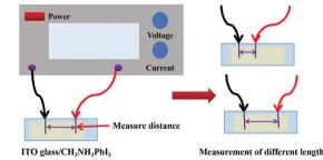
Fig. 10 Experimental scheme of resistance measurement for different CH3NH3Pbl3 perovskites.
