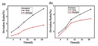
Fig. 12 (a) Absorption deviation ratio of different shaped CH<sub>3</sub>NH<sub>3</sub>Pbl<sub>3</sub> perovskites on different days and (b) resistance deviation ratio of different shaped CH<sub>3</sub>NH<sub>3</sub>Pbl<sub>3</sub> perovskites on different days.
