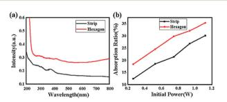
Fig. 9 (a) UV-vis spectra of two different shaped CH<sub>3</sub>NH<sub>3</sub>Pbl<sub>3</sub> perovskites and (b) absorption measurement of two different shaped CH3NH3Pbl3 perovskites, subjected to an incident laser with a wavelength of 468 nm.
