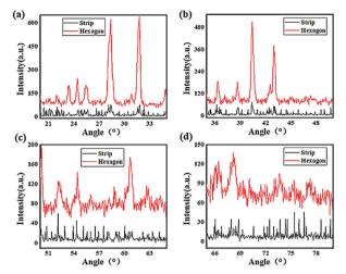
Fig. 5 XRD spectral analysis of different  $CH_3NH_3Pbl_3$  perovskites. (a) Diffraction angle range from 20° to 35°; (b) diffraction angle range from 35° to 50°; (c) diffraction angle range from 50° to 65°; and (d) diffraction angle range from 65° to 80°.
