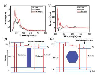
Fig. 7 (a) Emission spectra of different shaped CH<sub>3</sub>NH<sub>3</sub>PbI<sub>3</sub> perovskites; (b) excitation spectra of different shaped CH<sub>3</sub>NH<sub>3</sub>Pbl<sub>3</sub> perovskites; and (c and d) schematic illustration of the fluorescence mechanisms for different shaped CH<sub>3</sub>NH<sub>3</sub>Pbl<sub>3</sub> perovskites
