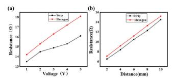
Fig. 11 (a) Resistance-voltage curves of the two different shaped CH<sub>3</sub>NH<sub>3</sub>Pbl<sub>3</sub> perovskites on ITO glass substrates and (b) resistances of the two different shaped CH3NH3Pbl3 perovskites on ITO glass, with the length of the ITO glass ranging from 2 mm to 10 mm
